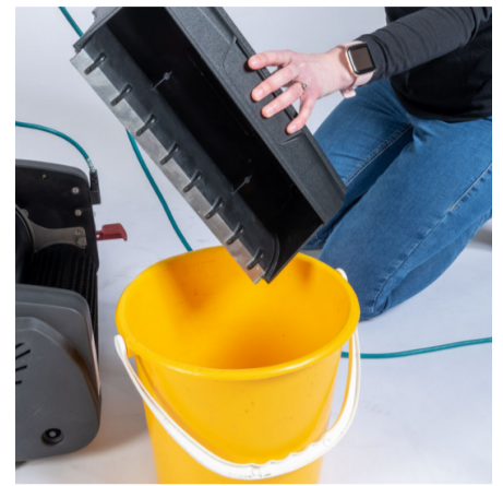
Once the machine has cooled down, remove, rinse and dry the recovery tank and replace.
