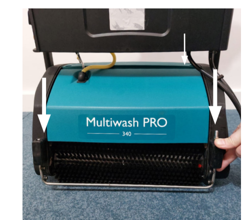
13 Slide the steam bar onto the front of the machine and position the steam shield onto the steam bar by locating the lower section to the steam bar first and then pushing the shield towards the machine.
