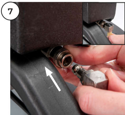
7 Connect the water feed hose into the solution tank connector.
