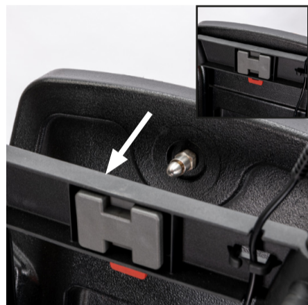
4 Position the solution tank into place, ensuring it hooks over the bottom handle and locks into position at the top of the tank.
