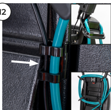
12 Feed the power cord through the cable restraint on the handle and wrap the power cord around the handle cord hooks.
