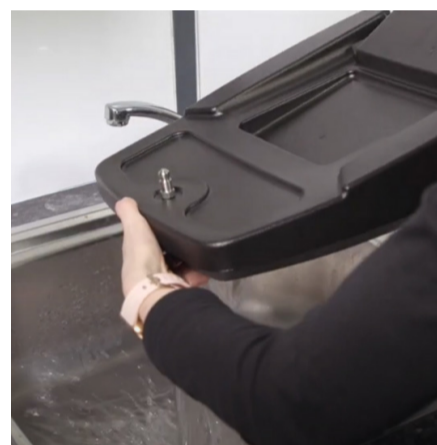
Remove, rinse with clean water and dry the solution tank. Replace the solution tank onto the machine and reconnect the hose.
