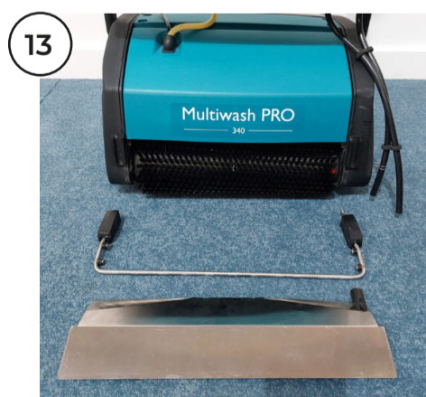
13 Slide the steam bar onto the front of the machine and position the steam shield onto the steam bar by locating the lower section to the steam bar first and then pushing the shield towards the machine.
